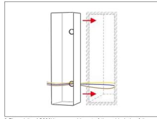
3.Thread the AC220V power cable out of the cable hole of the preburied box, and install the pre-buried box into the wall, flush with the wall, and fix it with screws.
