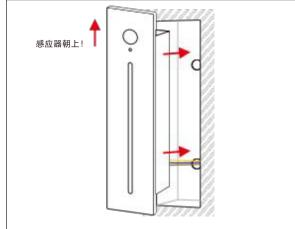
5.Install the lamp body into the embedded box and press it flat. Note: The sensor of this lamp is mounted upward!
