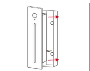
2. Separate the luminaire from the embedded box and remove the embedded box..
