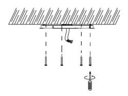
Install the mounting bracket onto the ceiling by using appropriately sized mounting screws and anchors. Ensure the screws and anchors used are suitable for the mounting surface and the surrounding environment.
