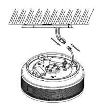
Connect the quick connector from the mounting bracket and the product together.
