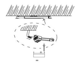
Loosen the nut and remove the cover from the terminal block. Connect mains supply wire to the terminal block. Ensure the wires are secure and no bare wires are exposed.
