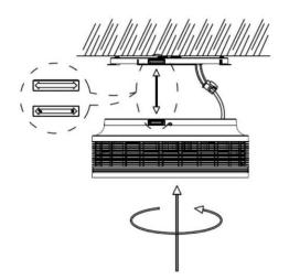
Install the product onto the mounting bracket by aligning the labels together and twist clockwise.
