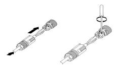
Connect the lamp power with driver power cable, and lock the waterproof connector
