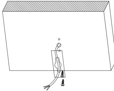
Fix the back cover of the bracket on the wall with two steel screw. Make sure the cable get through the hole in the middle of it.
