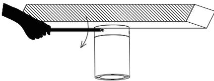
Fix the fixture on the back cover of the bracket with two screw.
