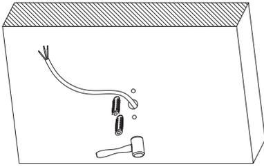
Drill two holes on the wall where you are about to install the lighting fixture. Then put two rubber plug into the holes respectively by using a hammer.
