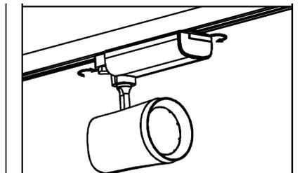
5. Plug the track wire into the socket and installation is done.
