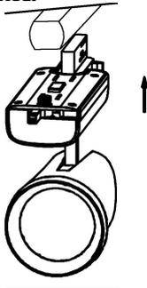
4. Turn the handles of the connectors 90° according to the illustrated direction and block the track light
