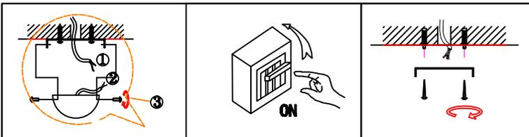
Connect wires according to below chart
