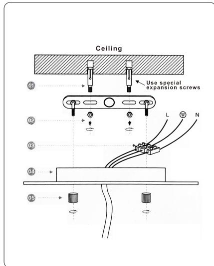
Installation diagram of ceiling lamp
